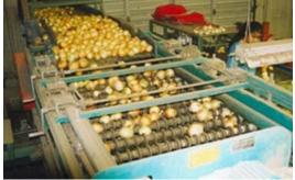
Fig.3.4.5 Sizing Rollers
