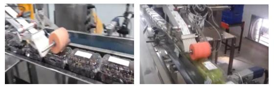
Fig.3.5.20 Automatic Labelling Machine
