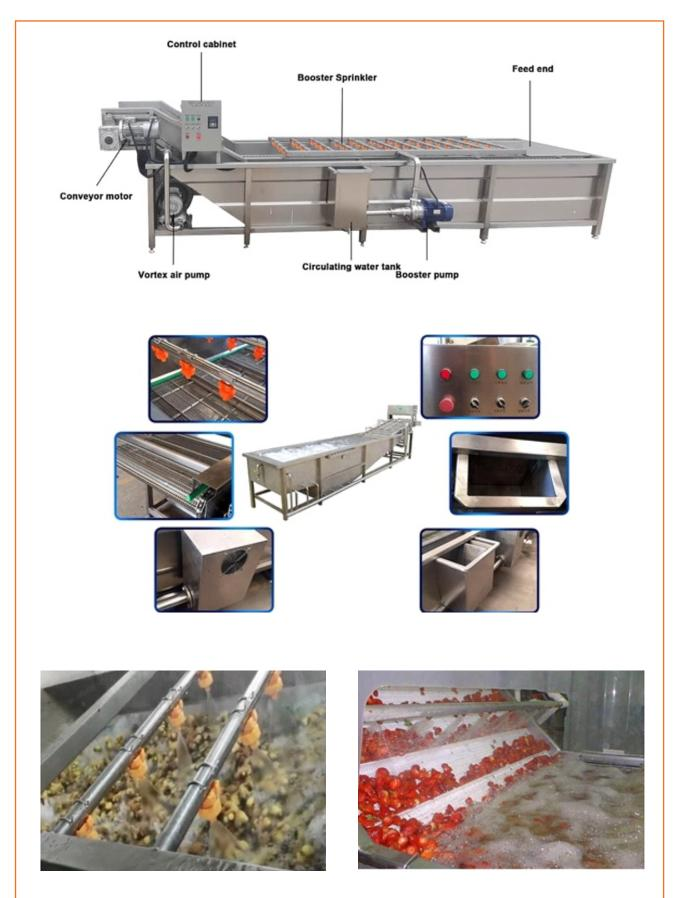
Fig.3.2.3 Air Bubble Washing Machine for Fruits and Vegetables
