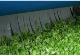
Fig.3.2.5 Pre-drying on a water removing belt and Air Drying Tunnel
