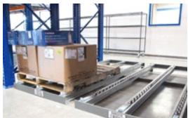
Fig.3.5.29 Pallet Flow Rack
