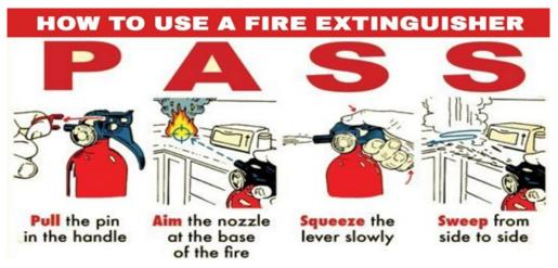
Fig. 5.8: Pass technique for Fire Extinguisher use
