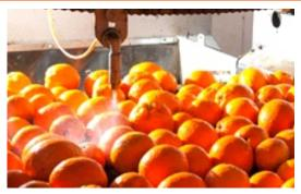
Fig.3.5.1 Spray Waxing using a Pump through low-pressure nozzles
