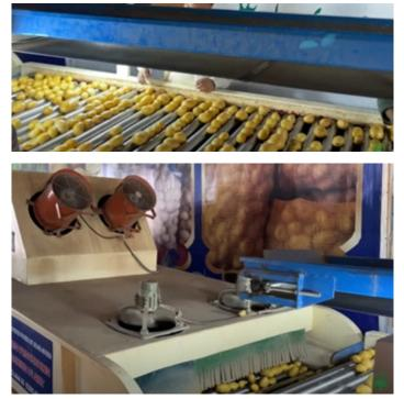
Fig.3.3.6 Drying Tunnel
