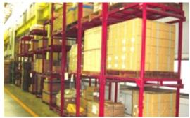
Fig.3.5.26 Stacking Frames
