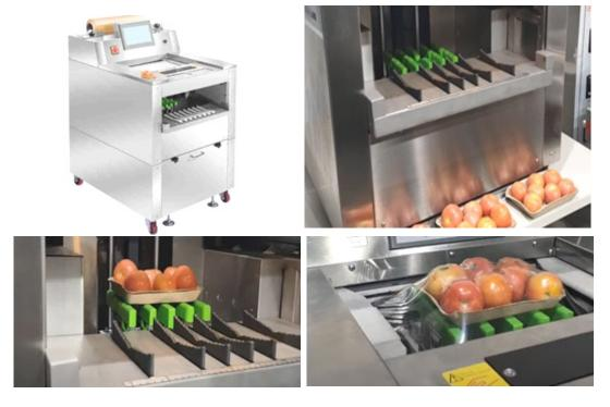
Fig.3.5.16 Cling Film Wrapping Automatic Machine
